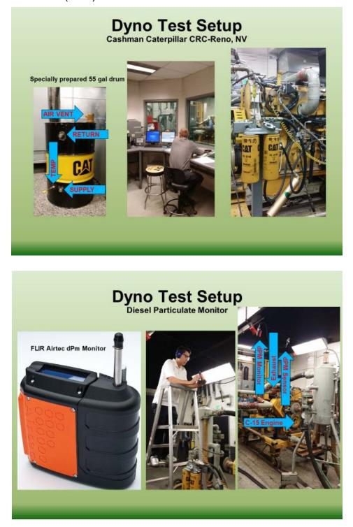
Test was conducted for Nevada gold mining subsidiary of large Canadian mining company. Fuel supplied from 55-gallon drum was pre-circulated through Fitch F150HDG (gold cylinder) in front of engine in 3<sup>rd</sup> photo from left above. FLIR Airtec dPm monitor is standard monitoring equipment for miners working in underground mines. Complies with NIOSH and MSHA standards for measuring dPm in real time.
